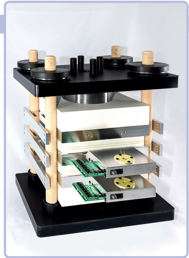
Example of stack with 5SNA3000K452300 IGBT modules
